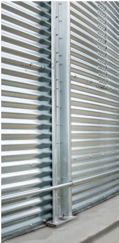
**G115 galvanizing** of stiffeners provides up to 27% longer life. Stiffeners are ASTM A653 Grade 55 with 55K yield and 70K tensile (except 18 gauge).
