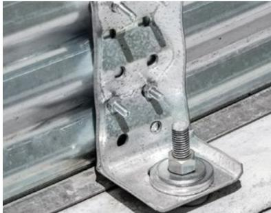
**Bin hold-down bracket** on 42' (12.80 m) to 60' (18.28 m) bins provides supplemental security and strength to one-ring base anchor.
