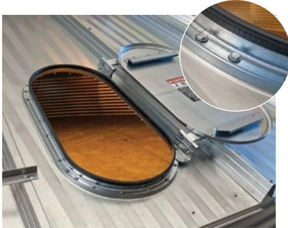
**Large pre-formed manway roof opening** is standard, featuring a hinged lid and big 5.5 sq. ft. (0.51 m<sup>2</sup>) opening for easy access. Easy-open lid with big beefy hinges lays flat to avoid wind. Seamless extruded collar (inset) with rubber gasket provides moisture-tight seal when closed. Pre-formed opening makes for simpler construction and tight fit.
