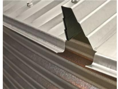
**Extra-tall 3-3/4" (9.5 cm) stair-stepped ribs** are staggered to provide even greater strength. Hemmed drip edge deflects moisture, eliminates sharp edges to reduce injury and strengthens the cross-section of the roof sheet.
