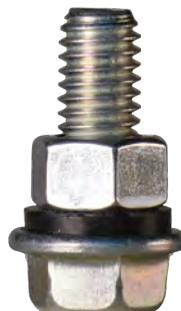
Top-quality fasteners feature JS1000 plating system, SAE Grade 8.2 for maximum shear capacity as well as industry standard washers to seal the bolt to the sidewall.
