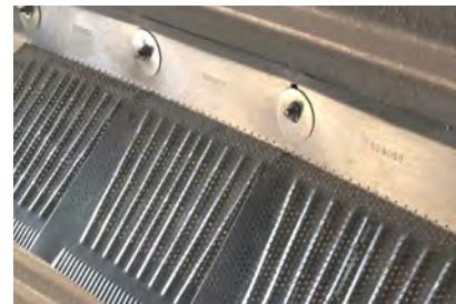
**Shedder plate**, supplied with all models, is a perforated component attached to the sidewall at an angle that matches the hopper cone angle. The shedder plate eliminates commodity hang-up were the sidewall connects to the cone.
