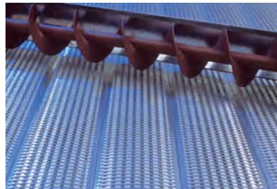
**Built-in crown on planks** prevents sagging and provides additional strength. Slotted design offers strength and economy.
