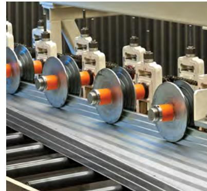
Proprietary state-of-the-art roll former controls the distance between holes from rib-to-rib, not from the edge of the coil like competitive products. The result: Higher quality roof sheets that fit better—with bolt holes that line up every time. Bolts drop right in place. That means trouble-free, labor-saving, frustration-free installation on site.
