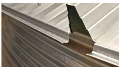
**Extra-tall 3-3/4" (9.5 cm) stair-stepped ribs** are staggered to provide even greater strength. Hemmed drip edge deflects moisture, eliminates sharp edges to reduce injury and strengthens the cross-section of the roof sheet.
