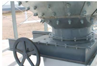
**Manual rack and pinion gate** controls flow from the tank and comes standard with all commercial hopper tanks.
