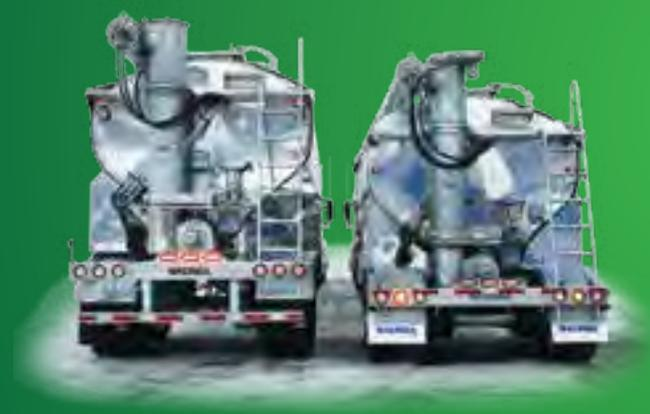
*Tanks are now lower to the ground and more stable to reduce rollovers. By reducing the height or lowering the centre of gravity, the unit is more stable.*
