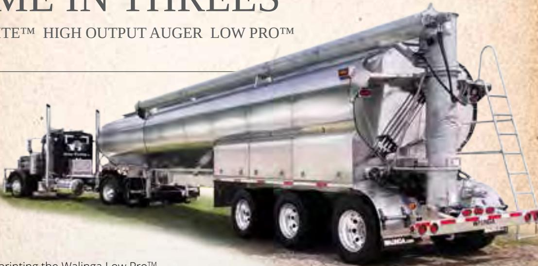
At the time of printing the Walinga Low Pro™, Ultra-Lite™ High Output Auger Unit (shown above) represents the state of the art in engineered transportation equipment. A proprietary variable thickness extrusion provides the spine for this all aluminum ultra light fuel-efficient design. Bulk is carried lower in the chassis, reducing wind resistance while lessening the risk of rollover. Add to that a Walinga high output auger transfer system and you have delivery efficiency without compromise.
